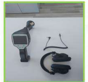
Periodic leakage control with compressed air leak measuring device
